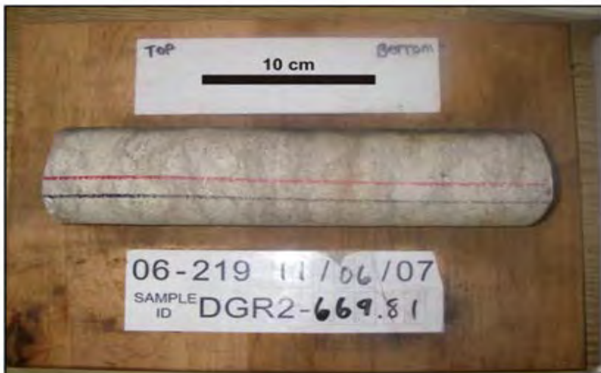
Figure 30: Core sample of argillaceous limestone from the repository horizon depth, Cobourg Formation, 669.8 meters below ground surface in borehole DGR-2. The limestone is dense with no visible pores, cavities, or fractures. (reproduced from DGR Geology TSD Figure 5.5.2-4)
