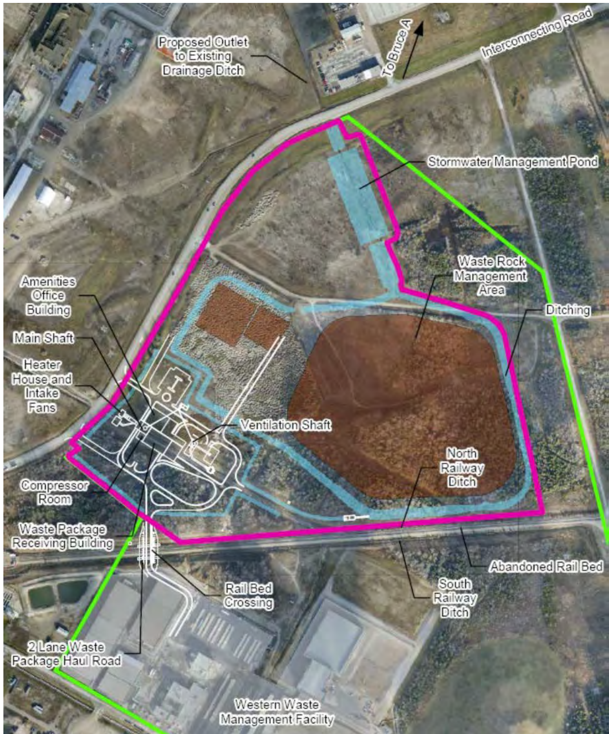
Figure 16: Site Drainage System and Surface Water Features (reproduced from CNSC PMD 13.P1-3I, Slide 15)
